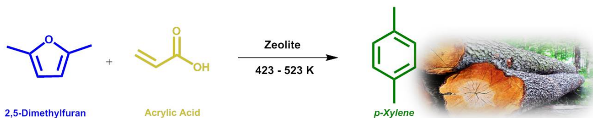
Scheme 1: Synthesis of p -xylene from cellulosic biomass-derived DMF and AA over different zeolite catalyst.
